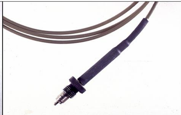
Close up view of output end after functioning showing firing pin protrusion
